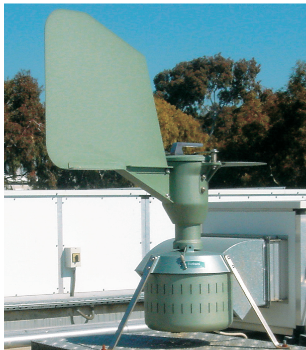
Figura 1. Polinómetro Burkard Figure 1. Burkard Pollen Trap
